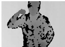
Figure: Noise in depth image
