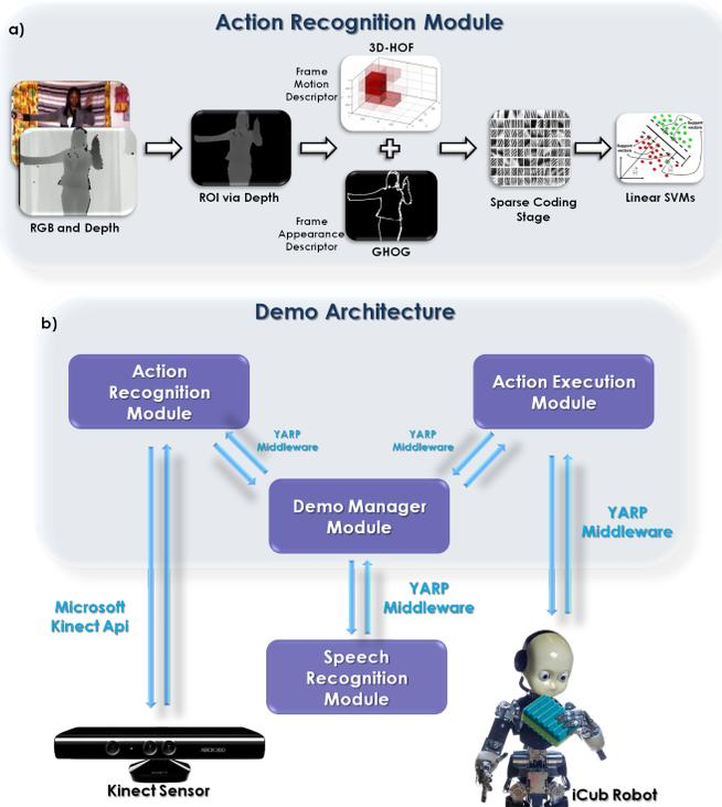
Figure 1. Fig. a): Overview of the recognition system. We propose a solution that cope with real-time requirements. Each frame is represented by 3DHOF and GHOG descriptors. The learning stage implicitly models the time dependency of actions concatenating descriptors of buffer of frames. Fig. b): Implementation of the demonstration. There are three main modules that take care of recognizing the action sequence, defining the game rules and making the robot perform gestures.
